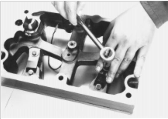
7. Make sure spring tabs are aligned with raised surface on end of piston.
